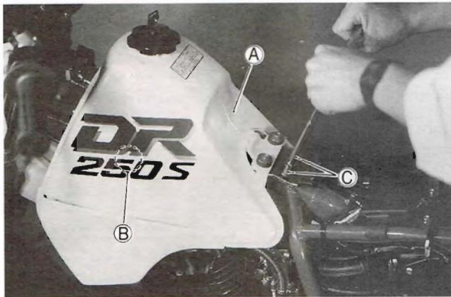
4. Fit the fuel tank mounting bracket to the cushion and install the fuel tank to the frame using two bolts.
