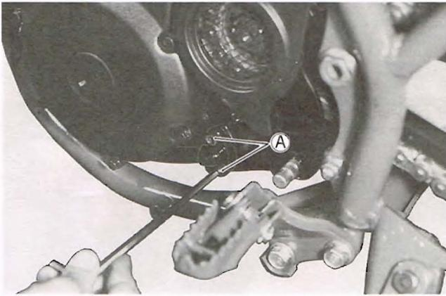
10. Remove the lower oil hose fitting bolts.
