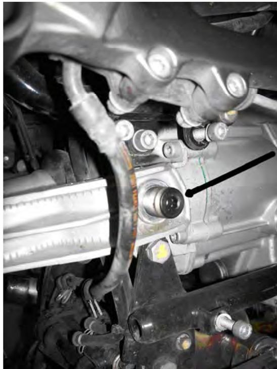
Remove the hose clamp that holds on the rubber boot for the universal joint. Remove the bolt that secures the bottom of the left-hand suspension unit to the swinging arm and voila! the swinging arm is no longer connected to anything.
