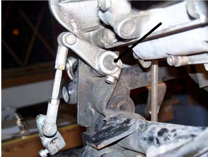
On the handlebars, remove the clutch lever pivot screw, line up slots on adjuster, slide out cable. Leave the whole mess hanging there, take the other end of the cable out of the lug on the top of the gearbox and disconnect the cable from the clutch operating arm.
