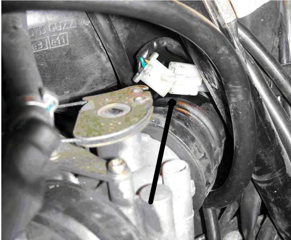
Remove the screw holding the two grounding wires to the clutch bell housing.
