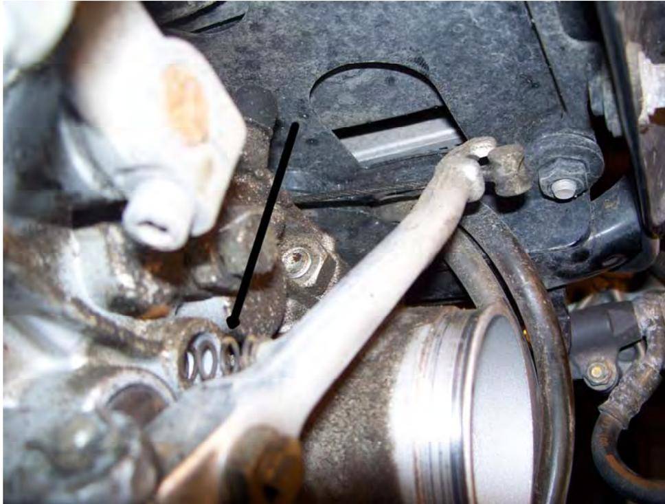
Remove the exhaust downpipes (they will come off as one piece with the expansion chamber, although they don't have to). Make sure you take out the gasket inside the head (5), behind the split collet (6). By the way, in the photo, the clamp (7) is upside down.
