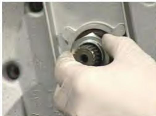
It appears from the parts list that a 'sieger' is an o-ring (Table 14, no. 14). If you kept the parts in order, it should be obvious. I can't remember; I hope I didn't forget it. And the 'blocking ring' is presumably the spacer that goes inside the oil seal behind the nut; it goes in tapered side first.
