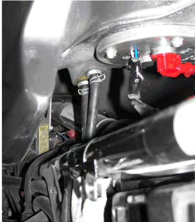
Disconnect the multi-pin connector (on the right-hand side) that goes to the fuel pump in the tank, and pull it up next to the red plastic elbow so that it won't get hung up on anything when you lift the tank:
