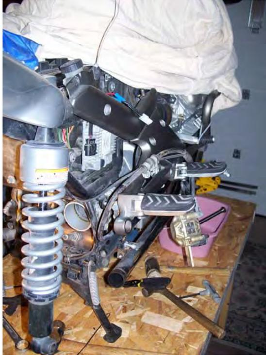
Unscrew the cover nuts and shouldered plugs on which the swinging arm pivots; mine came out much more easily than I thought they would.
