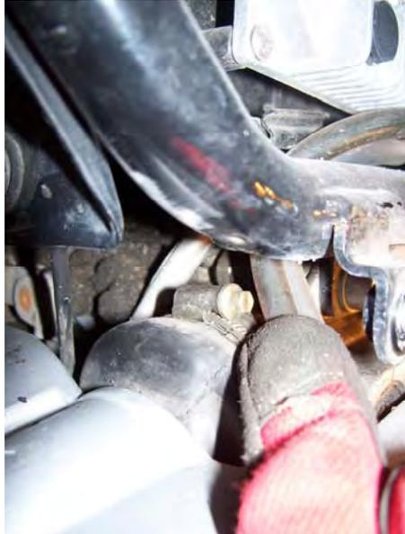
Remove the swinging arm. There's a thrust washer between it and the frame on the right-hand (drive) side, but not on the left, I have no idea why not.
