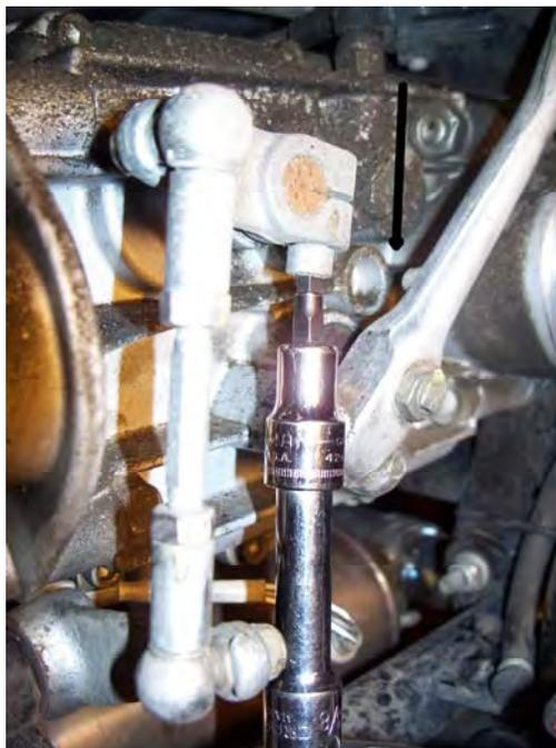
The arrow points to where the clutch arm return spring goes; this is the one you have to be careful not to lose when you disconnect the clutch cable.
