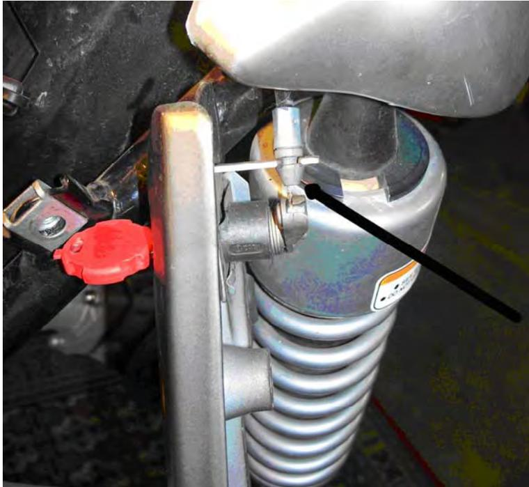
Remove the footrest mounting bracket from each side; on the left side you'll need to disconnect the seat release cable (picture). On the right side, leave the brake master cylinder right where it is, there's no need to detach it.
