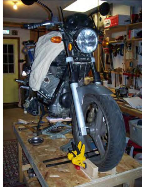
"There were some things I had to adapt because of the difference between the big block and small block Tonti frames. On our bikes there is a lower frame rail attachment that passes all the way through the timing chest. It is in the middle. On the big blocks, as described in the Roper pdf, you can pivot the frame on this bolt. I did not get that the bolt was in a different place on the small block until I had already started.
