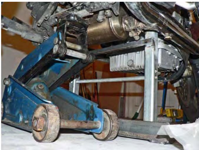
to put a jack or some kind of stand under the engine, it will prevent the bike from flopping about, since all that is holding it in place is the front wheel and the skyhook at the back.
