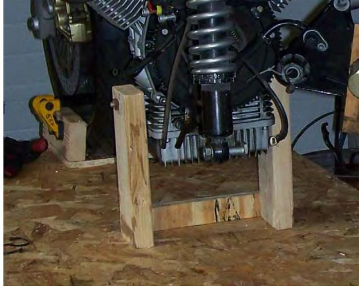
Or wait until the precarious arrangement of bits of wood on the jack falls over and the engine drops and gets jammed in the frame, and then build a stand that will hold the engine in place. Guess which one I did. If you used a trolley jack, it would probably be stable enough on that, but the jack would really get in the way; some kind of stand is more stable and easier to work round.
