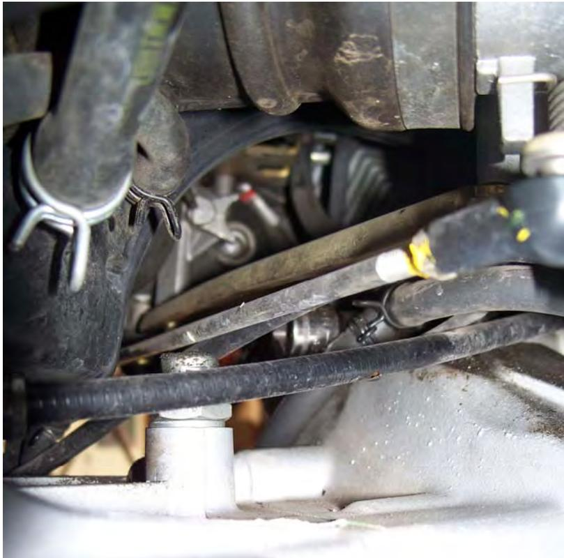
Muzz somehow got the Screw of Doom out without taking the throttle bodies off and without moving the engine; I could not do either, and believe me, I tried. There is simply no clearance; you can get a socket in (just) but not turn it.
