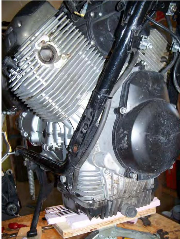
Remove the long through bolt at the bottom of the engine.
