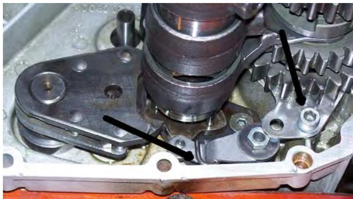
Next, refit the plastic oil tube, which has a notch that fits against the hex screw marked above, so you can't go wrong.
