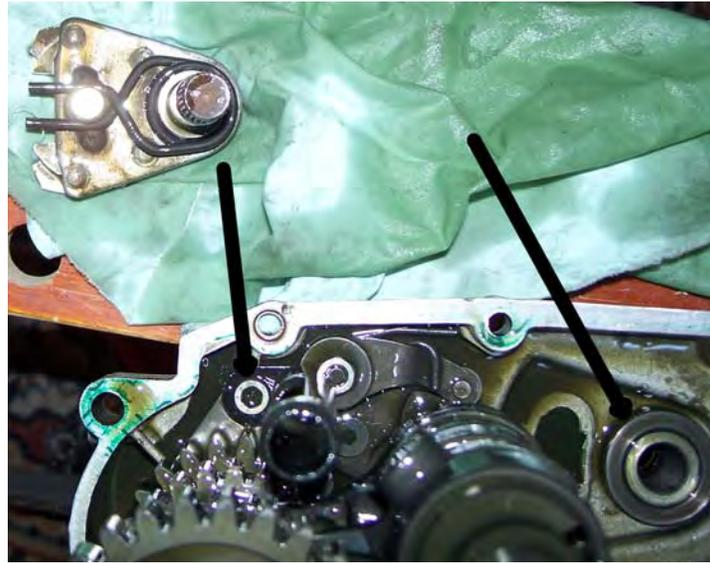
The 'blocking ring' (spacer, bushing) is still in place (right). Take care when passing the preselector shaft down the hole, there is an O ring there (barely visible).
