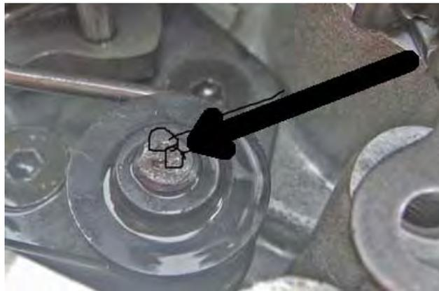
The stud was held at the two points marked, and the top of the stud, with the nut attached, was on the verge of going flying into the box, with spectacularly destructive results (not just for the bike – having your gearbox lock up solid is somewhere between frightening and fatal). Mine looked fine.
