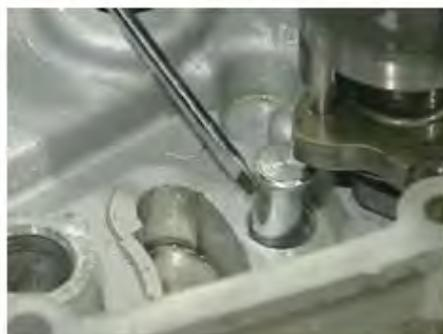
Not the clearest of instructions, but fairly clear from the picture: the solid side of the eccentric screw toward the pivot of the preselector. At that point the screw is in pretty much as far as it will go.
