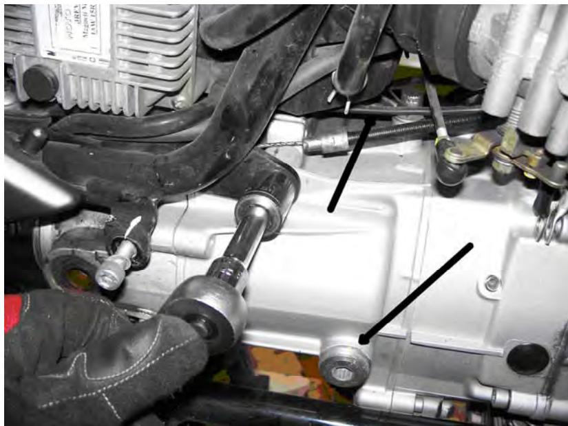
The arrows point to the gearbox filler/level plug and to what I think is the neutral switch wire. Once the gearbox is out, given that the neutral switch is so difficult to get at, maybe cutting the
