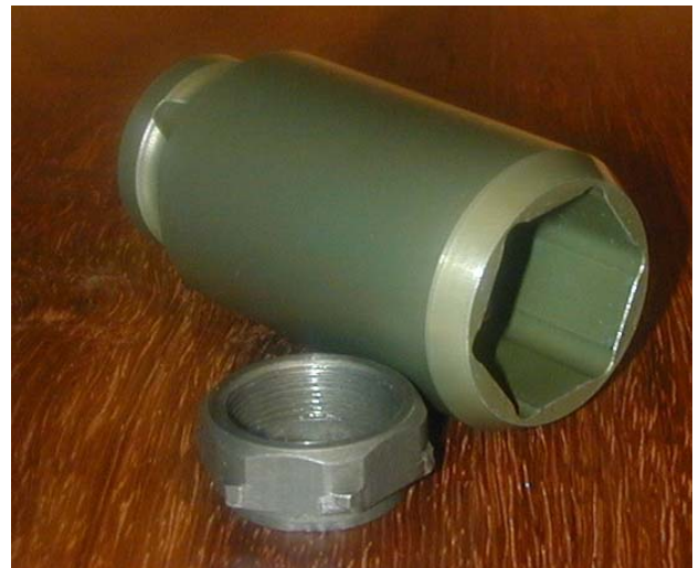
Fig.2 – Modified hex-pipe socket for the nut on the output shaft at the back of the gearbox
