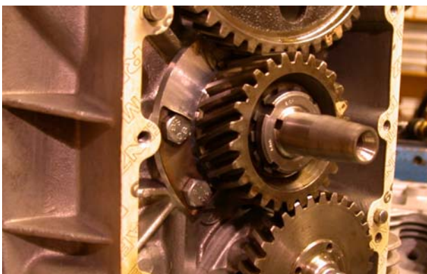
Fig.6 – Peg-nut at the front end of the crankshaft. (this is a Guzzi V7, i.e. without a timing chain, but with sprockets made of steel!)
