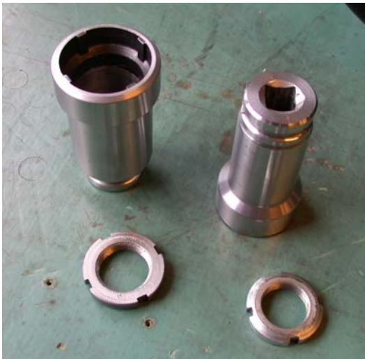
Fig.1 - Peg-nuts of two sizes, for the crankshaft (front) , and clutch boss on the gearbox respectively.
