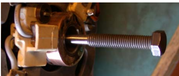
Fig.3 - Tool for pulling the alternator off the front of the crankshaft
