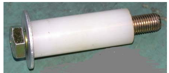
Fig.4 - Tool for centre-positioning and pre-stressing of the clutch on assembly
