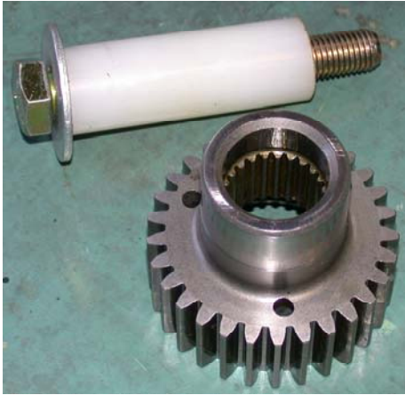
Fig.10 – Tool for pre-stressing and centre-positioning of the clutch, seen here with a clutch boss.
