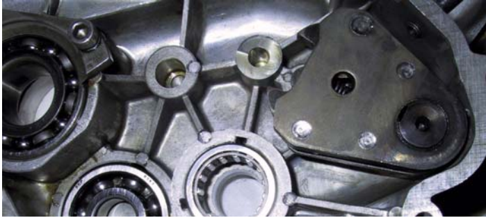
Fig.13 – The bearing on the output shaft (extreme left on the picture) seen from within the back lid of the gearbox.
