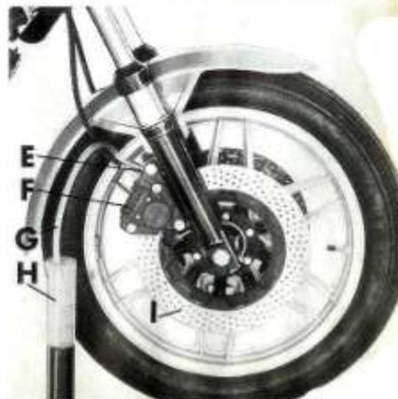
the aid of a suitable gauge and the reading should in no case exceed 0.2 mm (.0079"). If this «floating» is higher, it is well to ensure that the discs are properly assembled on the hubs, also the hub bearings play. The disc securing screws are tightened with a torque wrench set to 2.2 + 2.4 kgm (16 + 18 ft/lbs).
