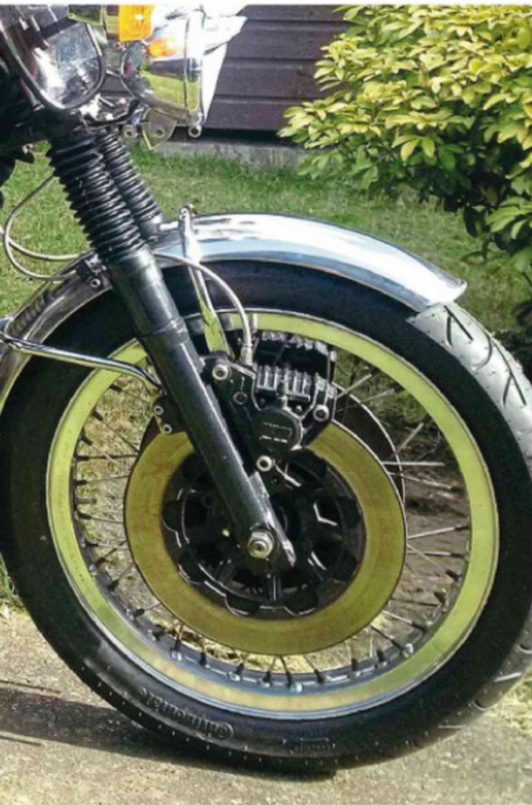
The twin discs and their linked actuation system make for arresting stopping
