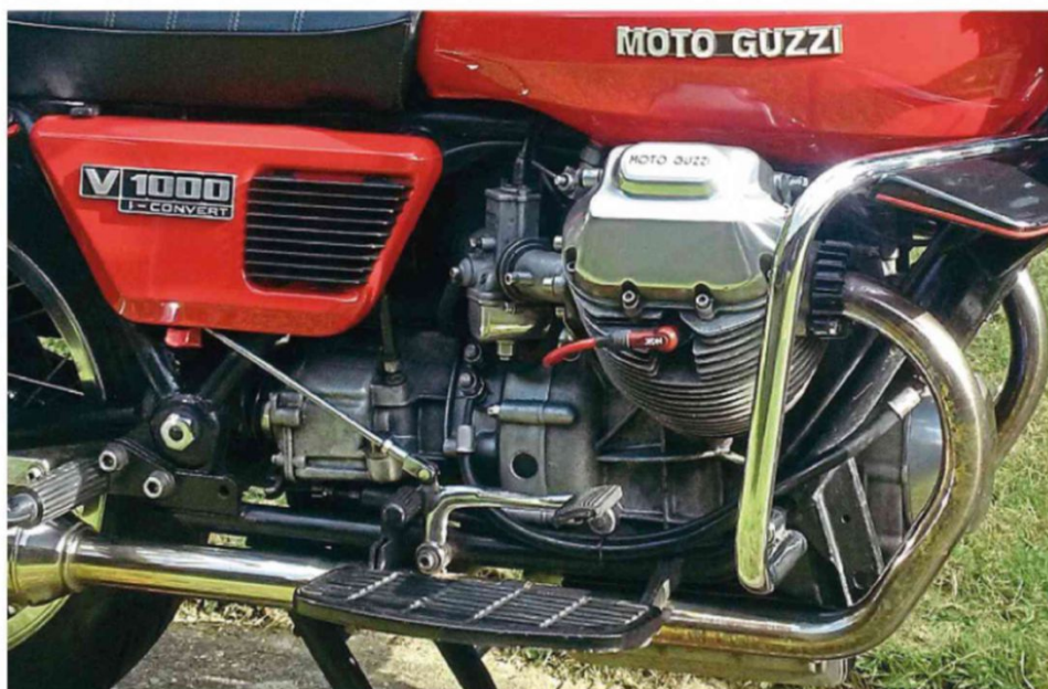
The rocker covers are custom jobs, ribs removed and polished up. The red HT leads may have been a momentary lapse of good taste
