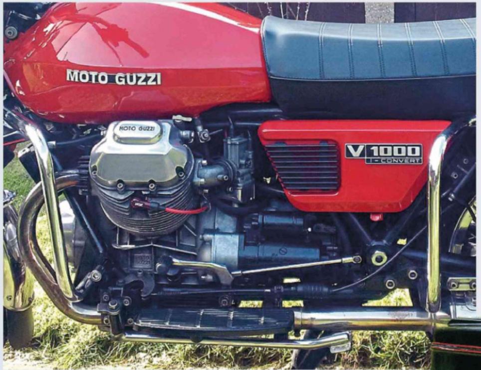
Garron removed the surplus-to-his-requirement 'heel' from the heel-and-toe rocking gear lever
