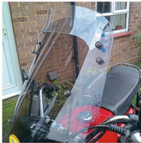
Tall riders can often suffer from excessive buffeting. Garron's answer was to fit a laminar lip to his Guzzi's windshield
