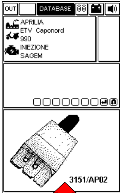
TYPE OF CONNECTOR TO CONNECT AXONE2000 SCAN TOOL TO ECU
