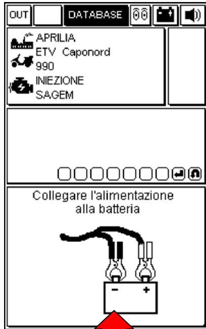
CONNECT AXONE2000 SCAN TOOL TO VEHICLE BATTERY
