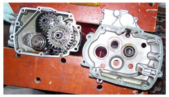
I have no idea why I have the gasket on the wrong section of the casing (right); obviously, it should be on the section with the gears in it (left), the way Signor GB has it, otherwise the gasket falls off when you lower the right section on to the left one.
