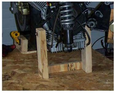
Or wait until the precarious arrangement of bits of wood on the jack falls over and the engine drops and gets jammed in the frame, and then build a stand that will hold the engine in place. Guess which one I did. If you used a trolley jack, it would probably be stable enough on that, but the jack would really get in the way; some kind of stand is more stable and easier to work round.
