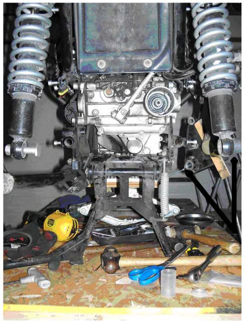
The arrows point to (a) wire tie holding bush in place in brake caliper. This is why you need lots of wire ties: not only are the bits together, you know which way round they go. Saves a lot of time and temper when you are putting the bike back together; (b) the rubber bush that you need a clamp and WD-40 to get back in, I wish I'd fixed it when access was this good. Live and learn.
