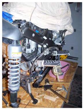
Unscrew the cover nuts and shouldered plugs on which the swinging arm pivots; mine came out much more easily than I thought they would.
