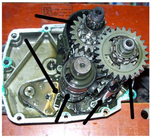
And there is the cause of the problem: jammed teeth on the preselector. It should not be possible for it to be in the position shown above.
