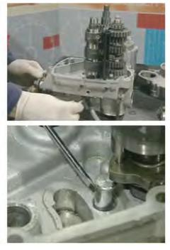
Not the clearest of instructions, but fairly clear from the picture: the solid side of the eccentric screw toward the pivot of the preselector. At that point the screw is in pretty much as far as it will go.
