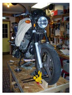
that this was developed for big-block Tonti-frame bikes, so needs considerable adaptation for use on the Breva. The basic principle is that, rather than leave the frame in place and move the gearbox and/or engine, you leave the engine and gearbox where they are and move the frame, pivoting it around one of the engine mounting bolts. This is how NOLAGuzzi described it:
