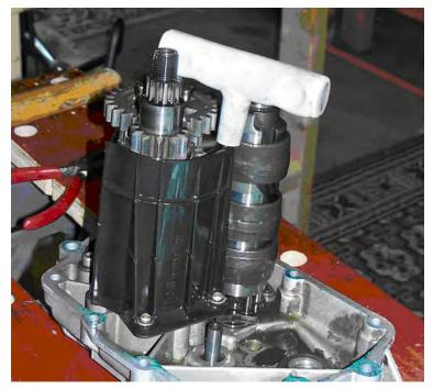
A longer key would be nice; I could only get about an eighth of a turn because the handle of the key hit the ends of the shafts. Once the screw is out, you will need something magnetic to fish it out with, unless you get lucky.
