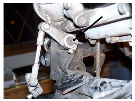
On the handlebars, remove the clutch lever pivot screw, line up slots on adjuster, slide out cable. Leave the whole mess hanging there, take the other end of the cable outer out of the lug on the top of the gearbox and disconnect the cable from the clutch operating arm.
