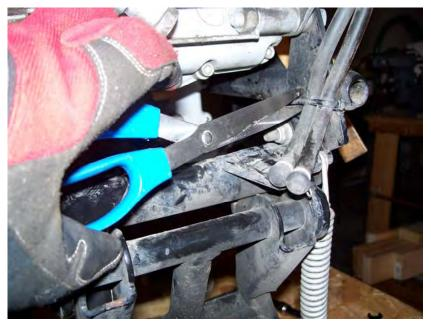
Off with starter motor. Nice and easy: two screws at the front, one fat wire, one thin wire. Like Muzz said, comes off quicker than a lizard up a drainpipe.
