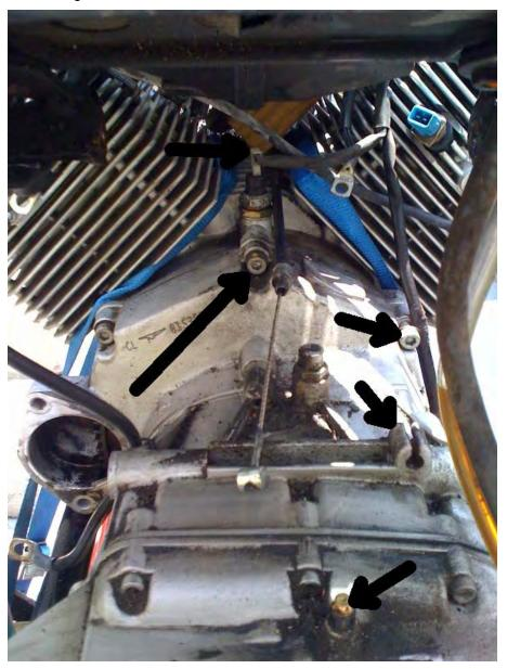
This is NOLAGuzzi's picture, showing (from the top, short arrows: oil pressure sensor, screw that holds both grounding cables, clutch cable lug, neutral indicator) and, with the long arrow, the Screw of Doom.
