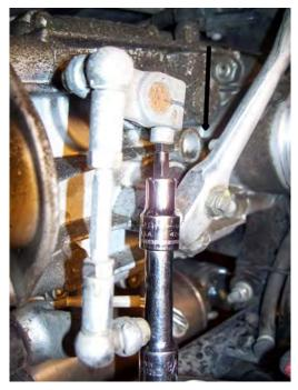
The arrow points to where the clutch arm return spring goes; this is the one you have to be careful not to lose when you disconnect the clutch cable.
