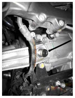
Remove the hose clamp that holds on the rubber boot for the universal joint. Remove the bolt that secures the bottom of the left-hand suspension unit to the swinging arm and voila! the swinging arm is no longer connected to anything.
