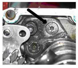
Although the access to this one is much better than for the previous two, it caused me more grief than anything else, including the Screw of Doom. I tried the hex key that got its neighbour out, but it felt like it might be slipping, so I ground the end off the key, the screw still didn't want to move.
