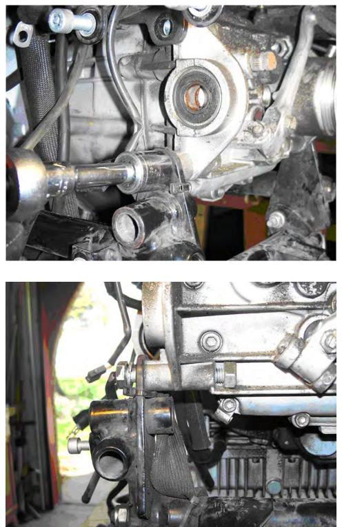
Jack the engine up ever so slightly, so that the jack, not the frame rail, is taking the weight. Remove the hex bolts connecting the lower frame rails to the front down tubes. Cut the wire tie first, obviously. You need to do this on the right-hand side only if you are using NOLAGuzzi's method or if you are skillful like Muzz and got the Screw of Doom out without having to move the engine.
