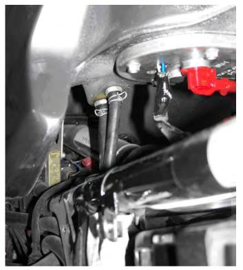
Disconnect the multi-pin connector (on the right-hand side) that goes to the fuel pump in the tank, and pull it up next to the red plastic elbow so that it won't get hung up on anything when you lift the tank:
