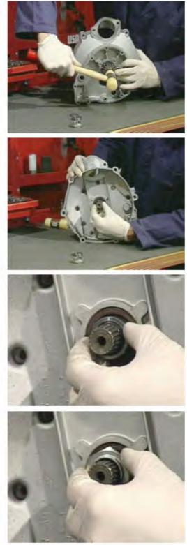
It appears from the parts list that a 'sieger' is an o-ring (Table 14, no. 14). If you kept the parts in order, it should be obvious. I can't remember; I hope I didn't forget it. And the 'blocking ring' is presumably the spacer that goes inside the oil seal behind the nut; it goes in tapered side first.
