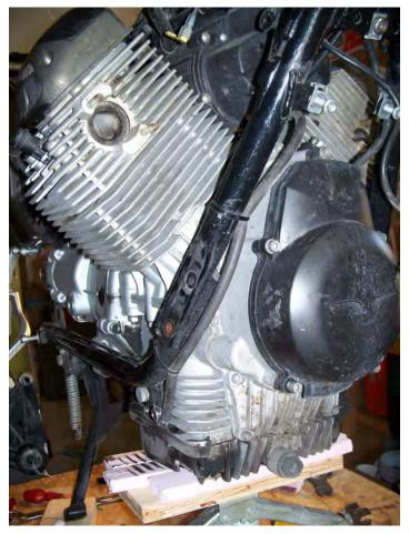
Remove the long through bolt at the bottom of the engine.
