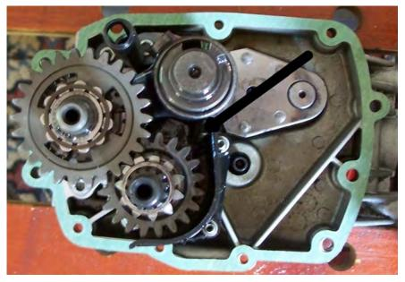
You need a hex key with a shaft at least 150 mm long. Mine came out fairly easily; Muzz' put up quite a fight. With this and the other two difficult screws, keeping downward pressure on the hex key while you get the screw free is important; sometimes it's best to put a ring spanner on the key and use that to turn it, while having one of the beer-drinking friends push down on the key.
