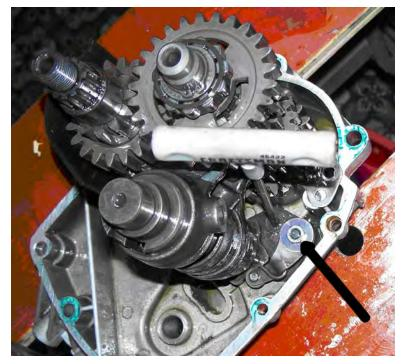
Next is the nut that holds down the spring-loaded arm that bears against the selector 'star'. The nut comes off easily, but when you pull the arm off its pivot shaft, the spring jumps out. No problem, you just need to be ready for it.
