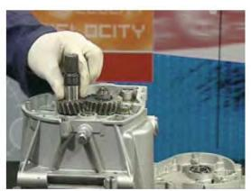
Insert the prescribed holding tool in the clutch shaft grooves
