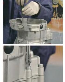
Tighten clutch shaft nut using the appropriate tool and stake.
