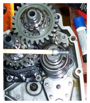
With a dab of grease on the washer to prevent it falling off the screw, you can then get the screw started in its hole way down there between the shafts, like so:
