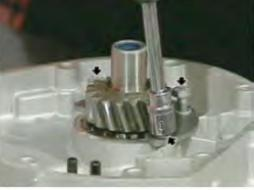
Position clutch housing gasket and place clutch housing in its seat.
