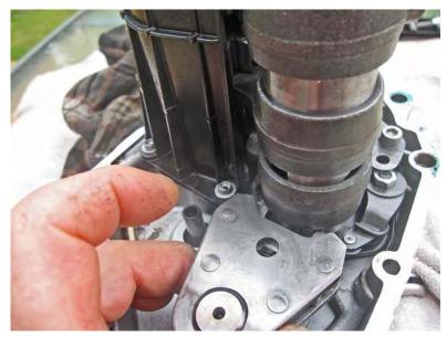
I managed to get mine out (just), but that was only because the teeth were jammed. Normally, you cannot get both teeth back that far; they are sprung in such a way that, if one of the teeth goes back, the other goes forward. Anyway, what this means is that you have to lift the selector drum so that you can get the new preselector fork in, and then get it to engage.
