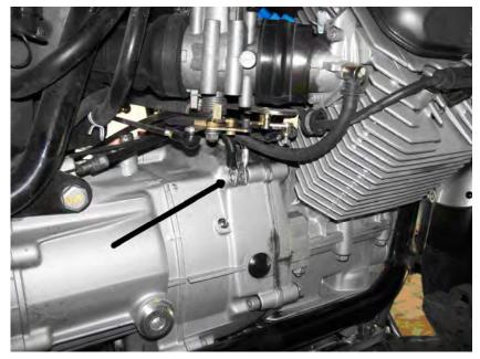
OK, back to the frame rails. This is pretty straightforward. Remove the black plastic guard in front of the sump. Support the engine with a jack (a trolley jack is best, believe me). Remove the lower gearbox mounting bolts.
