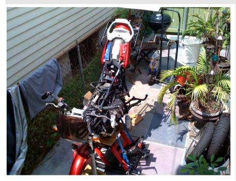
I pretty much followed the smallblock Breva frame manual on what to disconnect. I took off the entire exhaust system and then the tank. All of the electrical connections mentioned in the manual, pretty much everything except the oil sending unit. Next I started undoing all of the bolts (5, 10 and 7 in the picture) holding the upper frame to the gearbox.
