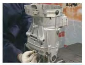
Insert clutch push rod in shaft with the greater diameter towards the control lever.
