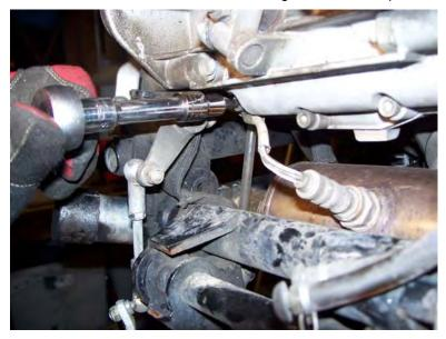
Disconnect the sensor cable at the connector:
