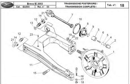
the pinch bolt and nut at the left-hand end (#16-18; 8-mm hex), and unscrew the axle (8-mm hex); a gentle tap with a hammer on the end of the axle helps to get it started. The spacer on the left will drop out, as will the brake caliper.
