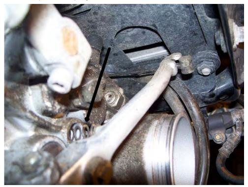
Remove the exhaust downpipes (they will come off as one piece with the expansion chamber, although they don't have to). Make sure you take out the gasket inside the head (5), behind the
