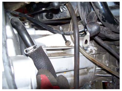
Disconnect the sidestand safety switch (you may not need to do this if you are taking only the right-hand frame rail off). There's a couple of wire ties that hold the hoses and wires to the frame tube, I'd cut them off by the time I took this picture. Obviously, they go where the hose is dimpled and/or there are marks on the frame.
