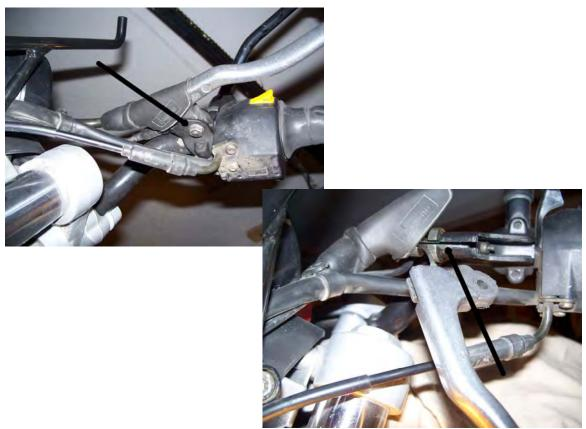
**WARNING WARNING WARNING:** The little spring under the clutch operating arm will go flying as soon as you release the clutch cable. Wrap a rag around it or put a cable tie through or have someone hold it or something, otherwise it will disappear and you will never see it again, at least not until after the replacement spring arrives:
