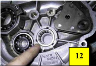
(Watch out for dropping needle rollers!)
