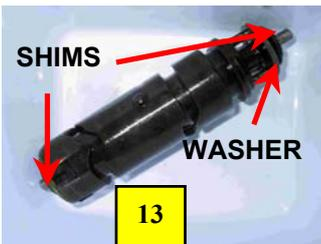
Having noted the position of the selector forks the selector drum can now be removed. Once it's out check to see if the shim at the front of the drum is still on the drum or if it's stuck at the bottom of the box. Wherever it is, retrieve it and slip it on to the end of the selector drum shaft and put the one from the back of the box on the other end and place the drum to a side for now (*p.13*).
