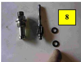
To start off with remove the speedo drive, being careful to remove the hardened steel washer (*see pic. 8*) from **under** the drive, **don't loose this**, you can't buy them separately!
