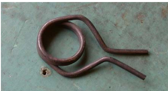
Fig.12 – Gear return spring (inexpensive part, known to have limited life)
