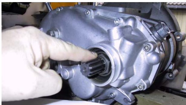
Fig.5 - Nut on the gearbox output shaft
