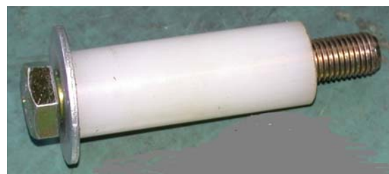
Fig.4 - Tool for centre-positioning and pre-stressing of the clutch on assembly
