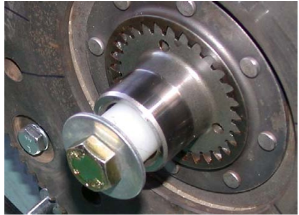
Fig.11 – Tool being used together with the clutch boss.
