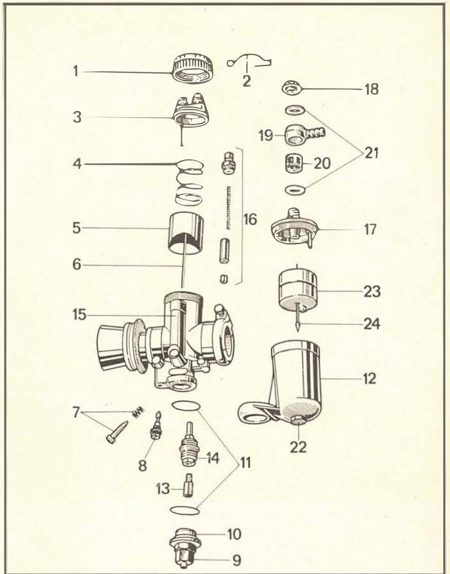
The V-7 has twin 29 millimeter Dellorto carbs, here is an expanded view.
