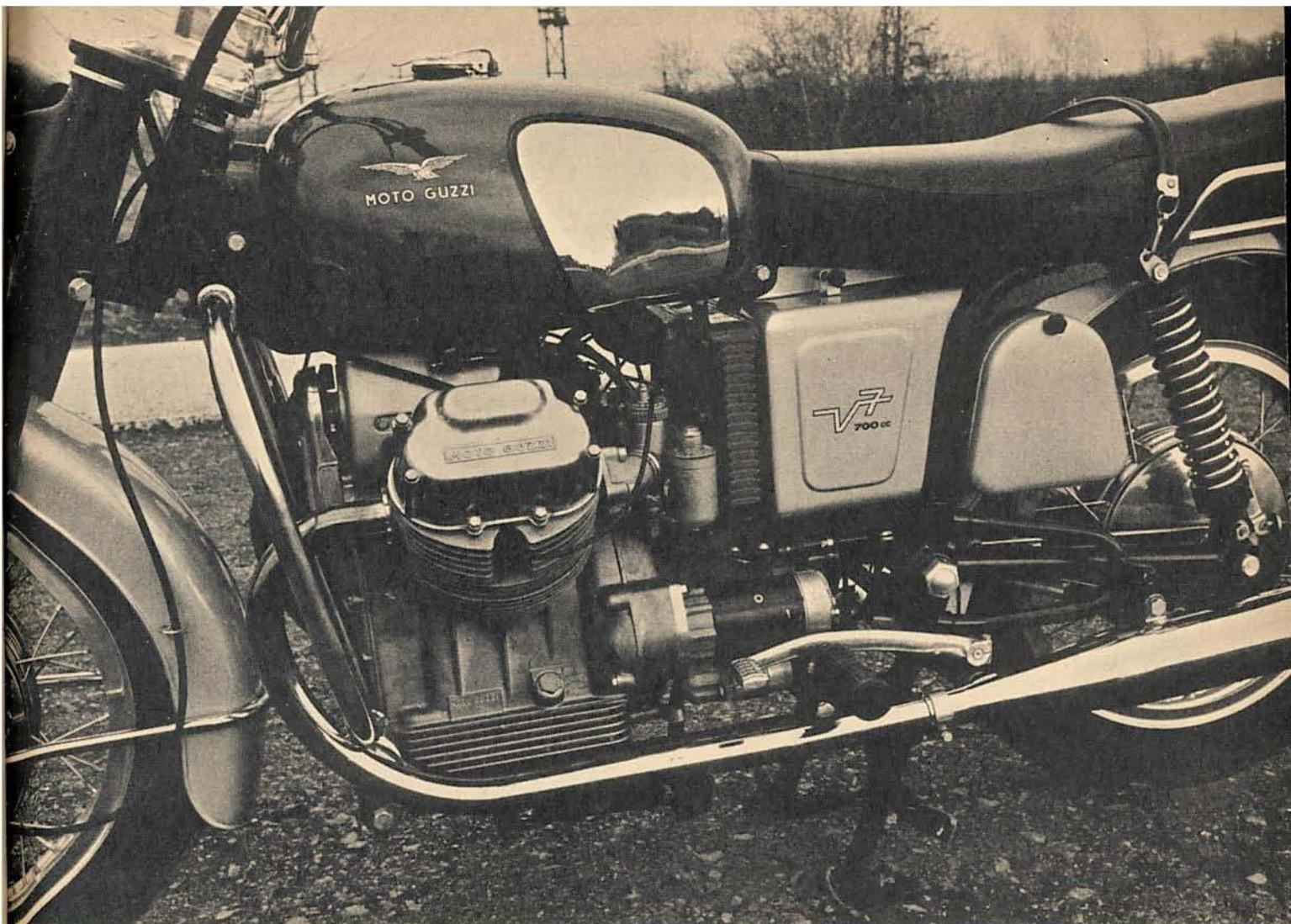
*The impression of the Guzzi is all engine; here you see why. Note the sump-finning and starter motor, also.*
