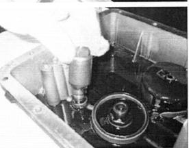
Disassemble oil overpressure valve, taking special care to keep the spring.
