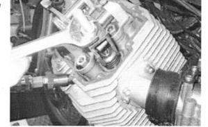
Using a mallet and the drift supplied with the tool for removing and installing the springs, gently tap to release the valve collets from the spring cap.
