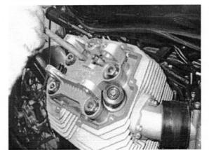
Remove the two rocker arm shafts.
