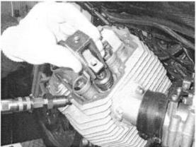
Bring the spring compression fork against the upper spring cap and slightly preload it by working the threaded pin.
