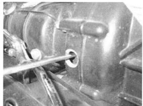
• Remove the stator locking nut, collect the spacer.
