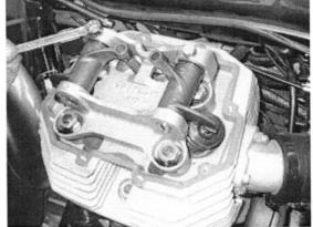
Fit the special tool part no. 03915530 (Tool for fitting and adjusting tappets) supplied with the kit.
