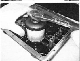
Loosen oil overpressure valve.
