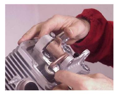
IF > 1.1 mm THE CLEARANCE IS CORRECT, LEAVE THE CALIBRATED PAD IN POSITION
