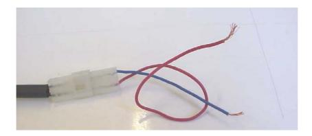
Connect a multimeter between the two wires and place the multimeter in  $\Omega$  mode (resistance measurement).
