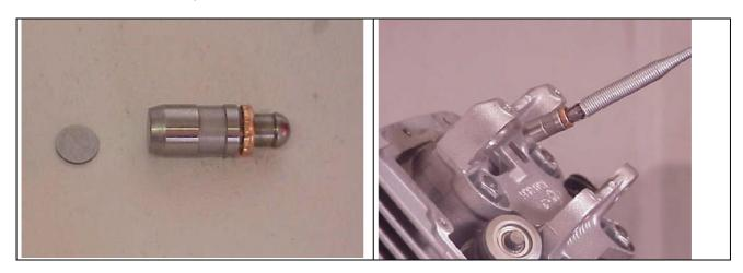
**5** FIT THE CLOSINGS, THE PADS AND THE **DRAINED** HYDRAULIC TAPPET INTO THE BLOCK; REASSEMBLE THE CAMSHAFT AND THE TIMING SYSTEM (GEARS-CHAIN-RODS-ENGINE MOUNT-ROCKER ARMS).
