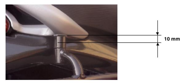
Should this minimum distance of 15 mm not be complied with, the bags could be damaged due to the heat produced by the exhaust fumes.
