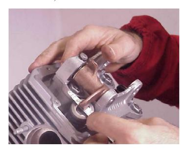
IF > 1.1 mm THE CLEARANCE IS CORRECT, LEAVE THE CALIBRATED PAD IN POSITION IF < 1.1 mm REMOVE THE CALIBRATED PAD (USE A MAGNET; SEE PHOTOGRAPH)
