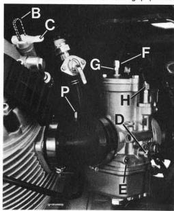
the slides have the same opening. If not, undo locknuts "G" and act on adjusters "F".
