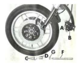
Jean the vehicle to the right just sufficiently to allow the wheel to be withdrawn from the rear fork arm and the rear drive box.
