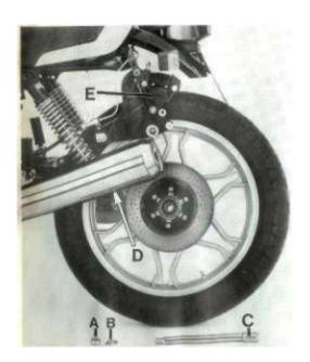
To re-assemble, reverse the dismantling sequence, remembering to insert the plate complete with caliper on the stop lug on the left arm of the swing fork.
