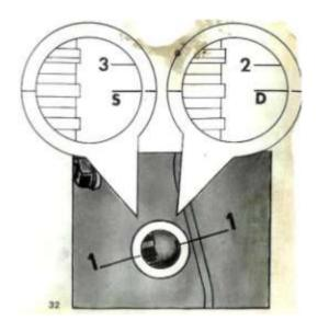
46 • now rotate the flywheel clockwise until mark «3» (fixed advance) coincides exactly with mark "1,, on the inspection hole rim. At this point, contact points of breaker «B» "B" fig. 31) should start to open.
