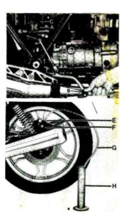
28 plug «E». remove plastic duct "G", and re-fit rubber cover on the drain plug. If the air bleeding operation has been carried out correctly, a direct and efficient working of the fluid will be perceived immediately after the initial idle movement of control lever "8". If not repeat the operation until the above result is achieved
