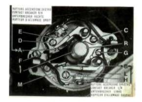
Checking and adjusting the ignition timing "fixed advance •• (fig. 32)
