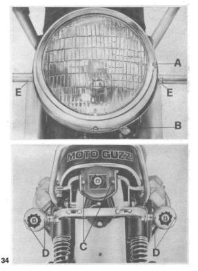
55 By re-fitting of reflectors screw in uniformly, do not lock screws too much to prevent braking of same.
