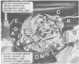
After setting the correct distance, lock screws «C» and «D».
