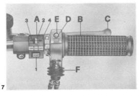
16 Engine starting and emergency stopping (fig. 7 «A»)
