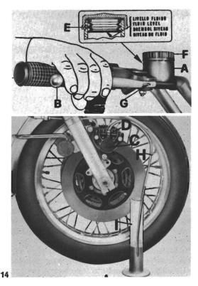
Adjusting the front brake (right) control lever (fig. 14)
