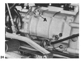
36 This operation should be carried out a short time after a ride when the oil is still warm and easily drained.
