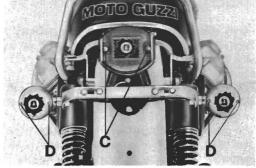
52 By re-fitting of reflectors screw in uniformly, do not lock screws too much to prevent braking of same.
