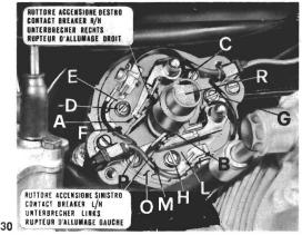
After setting the correct distance, lock screws  ${\rm eC}{\rm s}$  and  ${\rm eD}{\rm s}.$
