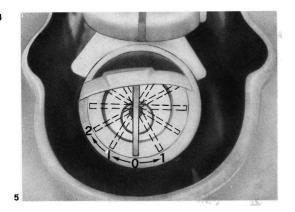
out when the pressure is sufficient for normal engine lubrication. Should it not go out, the pressure is not correct; in this case the engine has to be stopped and suitable checkings are to be carried out.
