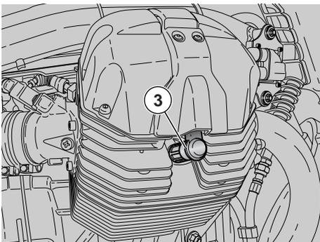
Periodically remove the outer spark plugs (1), clean scaling and change, if necessary.
