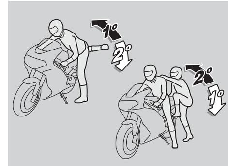
**NOTE** The rider must get on the vehicle first and get off last to ensure he/she has control and balance of the vehicle while the passenger is mounting or dismounting.
