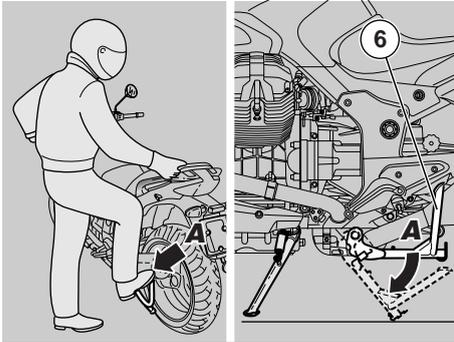
**NOTE** Do not rest the side stand to ground. Keep the vehicle upright.
