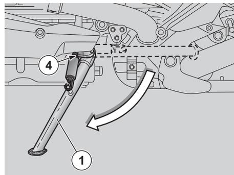
The side stand (1) is equipped with a safety switch (4) that inhibits ignition or stops the engine whenever a gear is engaged while the side stand (1) is down.
