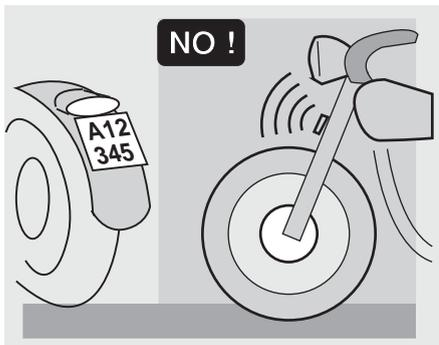
Never change the position, inclination or colour of: number plate, turn indicators, lights and horns.
