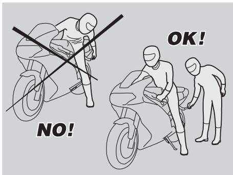
When getting on and off the vehicle, the passenger must move carefully to avoid causing imbalance.
