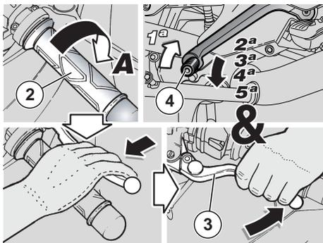
When the vehicle is at standstill with the engine running, avoid keeping the clutch pulled with a gear engaged for a long time or the clutch will overheat.
