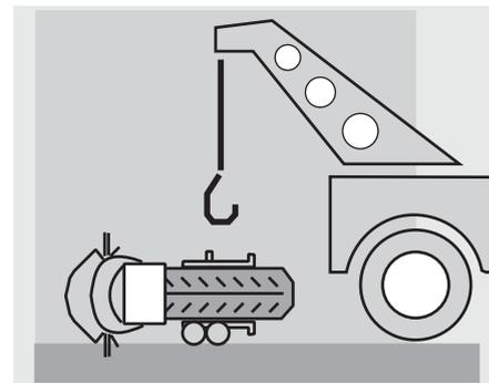
If the vehicle has been involved in an accident, check the control levers, pipes and hoses, wires, the braking system and key components for damage.
