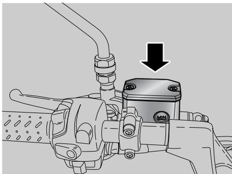
The clutch reservoir is located on the left handlebar, close to the clutch lever fitting.
