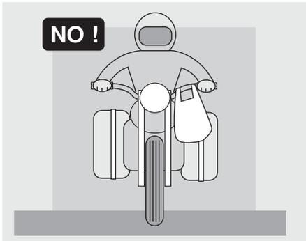
Avoid fixing bulky, heavy and/or dangerous objects to the handlebars, mudguards and forks - this could slow down the vehicle's response in turns and would inevitably affect handling.
