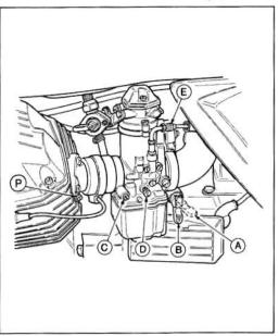
the slides have the same opening. If not, undo locknuts and act on adjusters.
