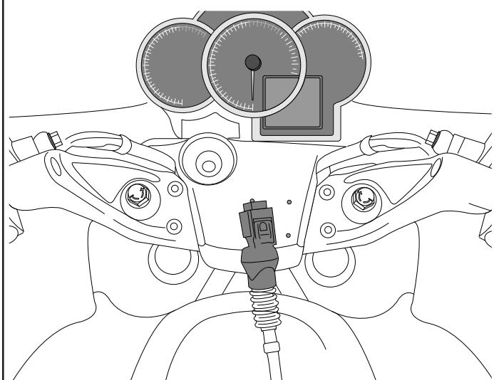
**GB** Remove plate cover unbolting **C** the two screws **D** showed.
