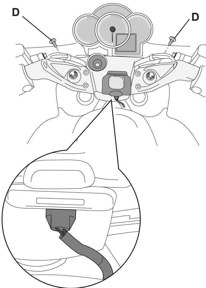
**GB** Refit steering plate cover using original screws **D**.
