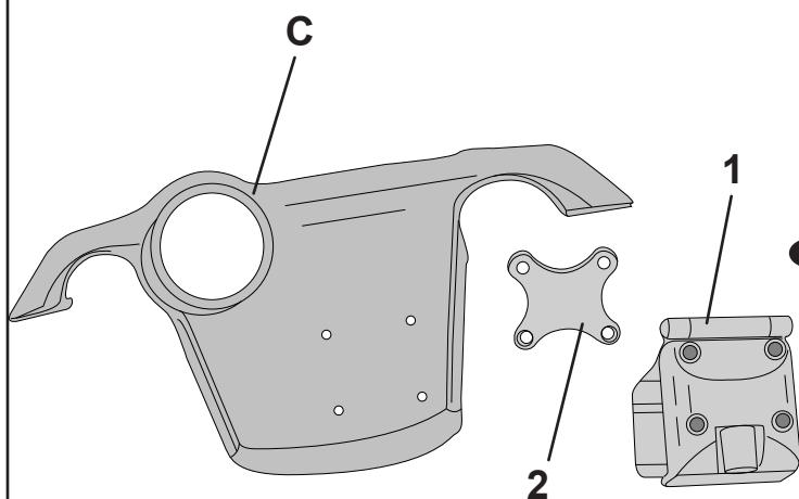
**GB** Assemble navigator support contained in the TomTom 1 kit as well as the cover for the steering plate **C** inserting the black plastic hold **2** provided with the kit.
