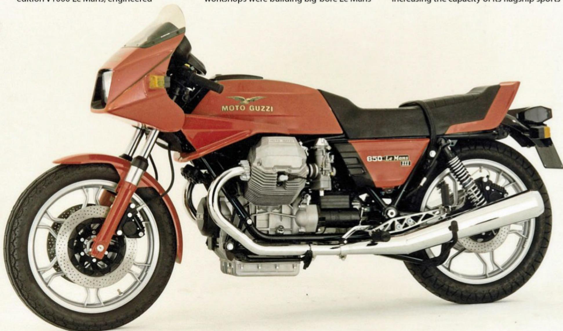
bike, retaining the 850's bore and stroke of 83 by 78mm. Angular covers and plated exhausts capped the restyle, which was shipped worldwide for 1982.
