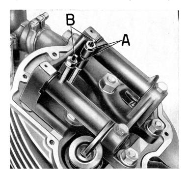
allow the cylinder head to be withdrawn, take off the carburetor, exhaust pipe, rocker box, rockers and the 4 hold down nuts.
