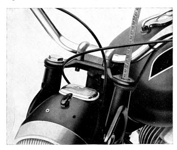
is recommended to clean the filter in the banjo union (A in fig. 17) with petrol or an air jet. Access to this filter is obtained by unscrewing the top nut.
