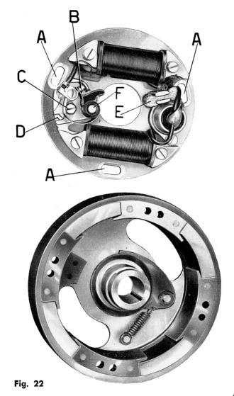
will be necessary to remove the flywheel rotor and to shift the stator to a position where the points start opening correctly. Slacken the 3 screws which hold down the stator. To do this see A in fig. 22.
