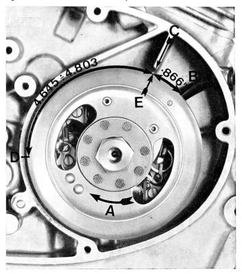
check whether the contact breaker points are correctly set at 0.4 mm. (.0157"). Place now a piece of tissue paper between the points and turn the flywheel anticlockwise till the paper is firmly gripped.
