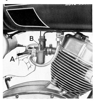
Needle B 10, second notch from top. In very cold weather, it is advisable to raise the needle one notch.
