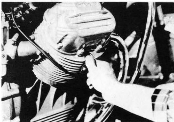
1. Remove sparkplug wires by pulling out and twisting gently. Do not jerk plug wires as damage may result causing replacement of plug wires
