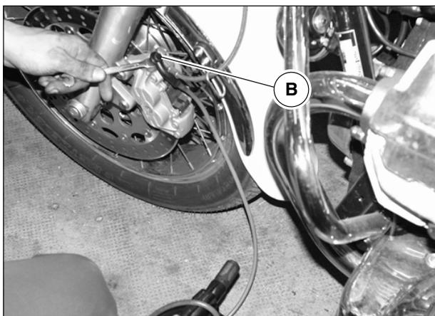
If no drainer is available, connect a small transparent plastic tube to the draining union, as described for draining the system.
