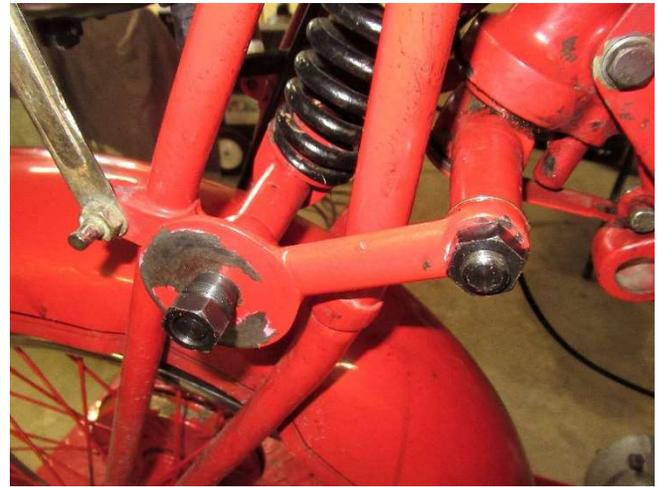
Nuts tightened on left lower link to check endplay.
