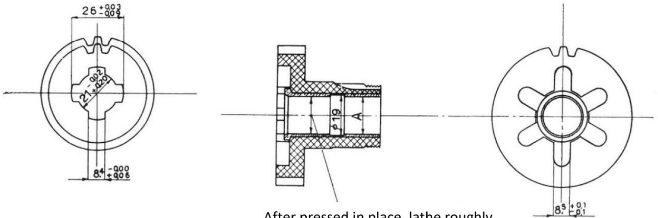
After pressed in place, lathe roughly to 18,5 +/- 0.02 then ream precisely to 18,58 +/- 0.01.
