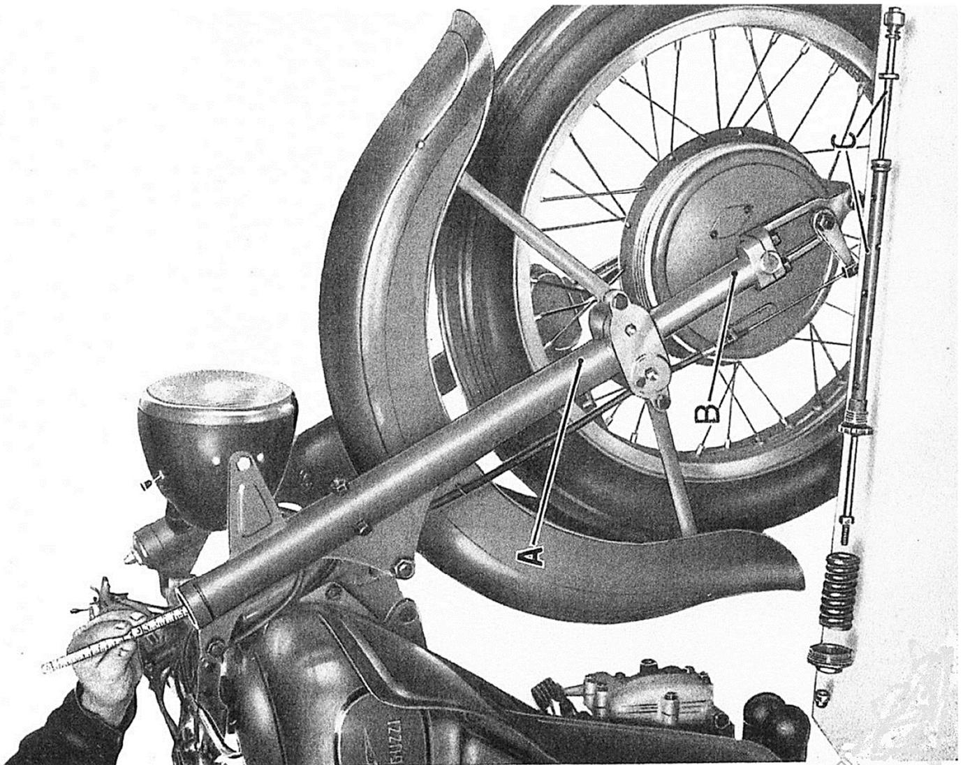
Figure 34- Verification of the liquid in the telescopic fork.
