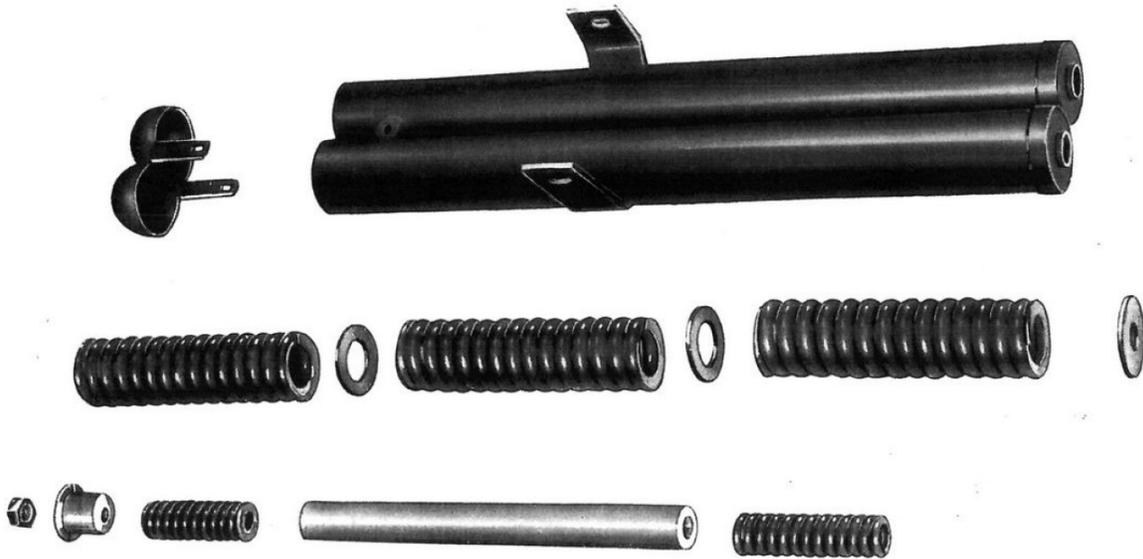
Figure 31- Springs and carrier tubes: notice the group is removed from the suspension.
