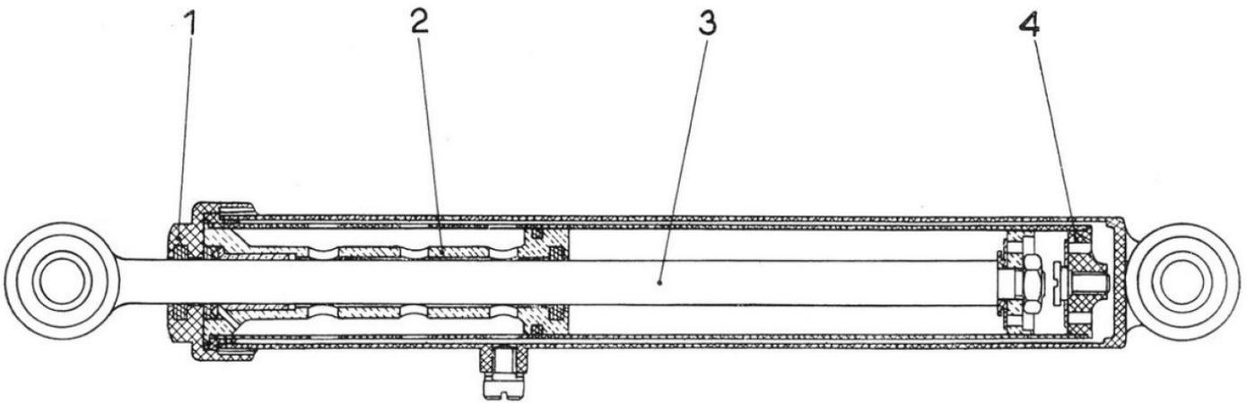
Figure 33- Internals of the rear dampers.
