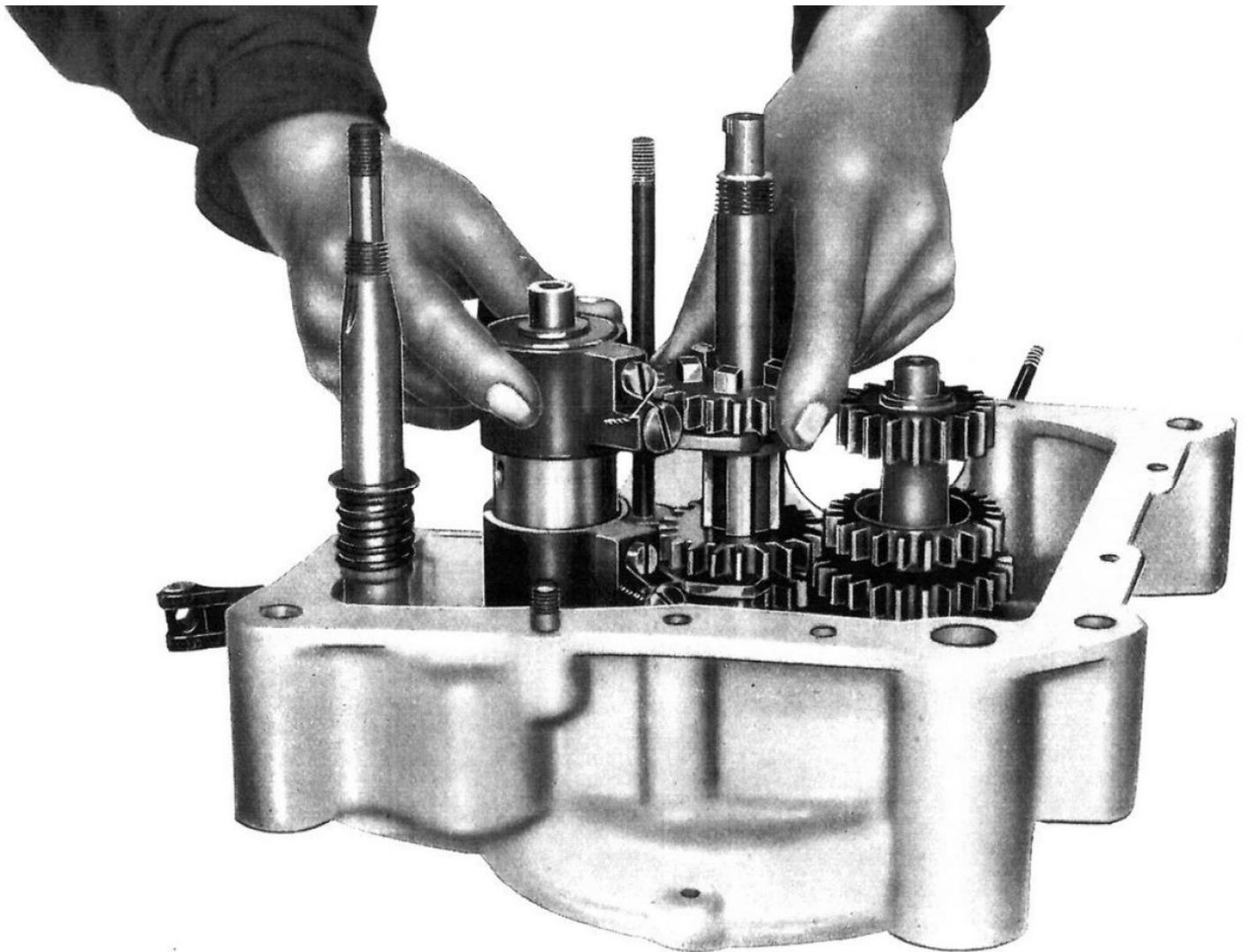
Figure 22- How you must assemble the gear change into the left half of the crankcase.
