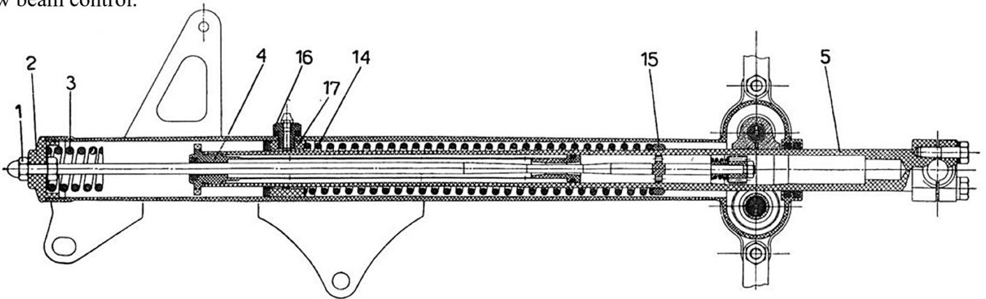
Figure 32- Internals of the telescopic fork.
