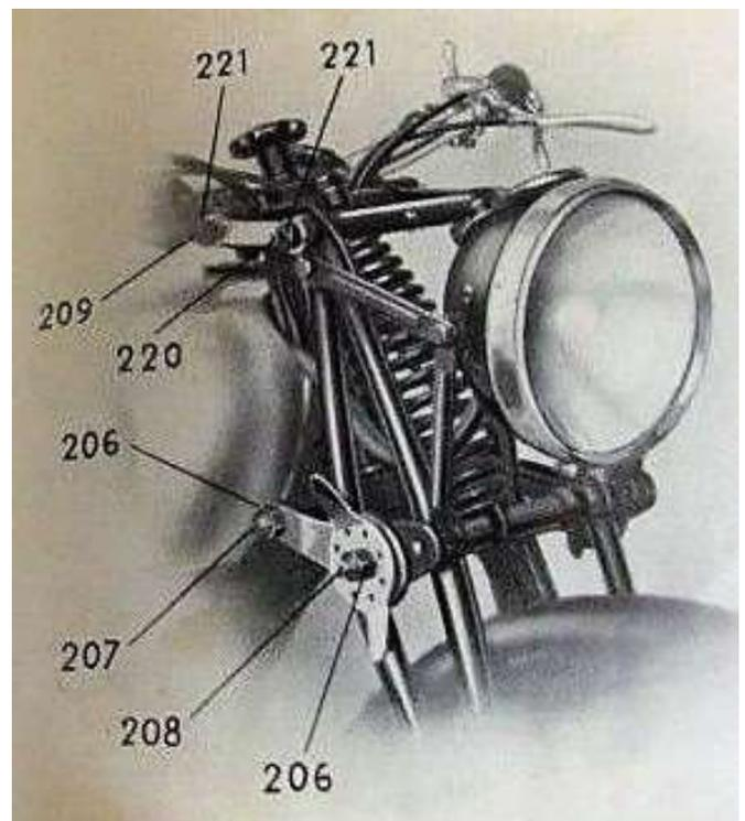
the long edge of the square against the pivot eyes and compare the alignment to the ends of the straight rods. Side links are straight with both ends of the link in the same plane (in other words the thickness of the bronze washers should be the same at both ends of the link.). Upper links are 8 mm thick at pivot pin eyes. Lower links are 11 mm thick at pivot pin eyes.
