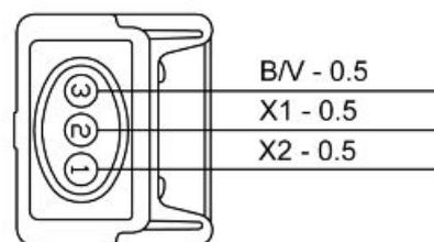
3. Engine speed sensor anti-jamming cable
