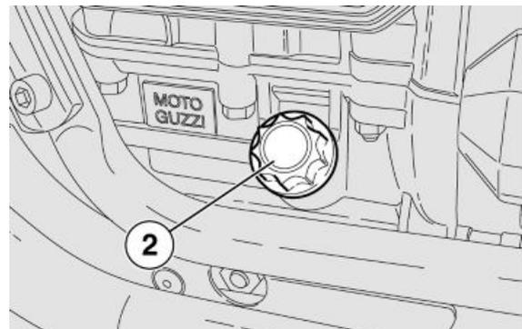
**Drainage plugs tightening torque (1): 12 Nm
