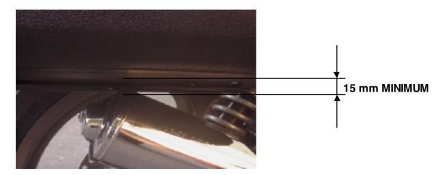
If this distance is shorter, it is possible to lift the bag attachments by shortening of 10 mm the bushes placed between the attachments and the bike frame.
