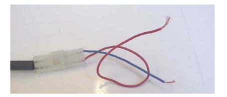
Connect a multimeter between the two wires and place the multimeter in  $\Omega$  mode (resistance measurement). The resistance should be 33±2  $\Omega$
